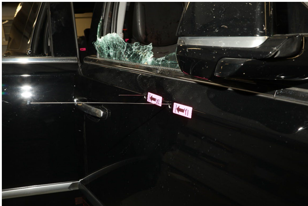
Trajectory rods showing entrances of bullet paths X and Y
